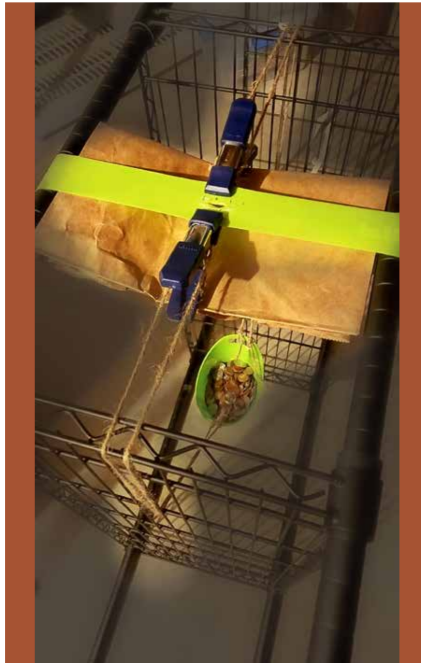
James, in Lt Col Maffei's basement, has reconfigured a shelving unit to test the adhesiveness of Derma-bond in test and control samples
