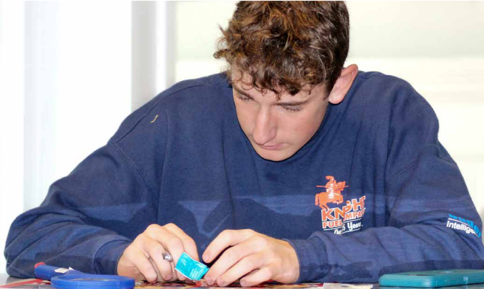
Tommy is making a criss-cross cut on each of two contact lenses. Will the fluorescein dye from the control and flight samples be able to pick up the scratches?
