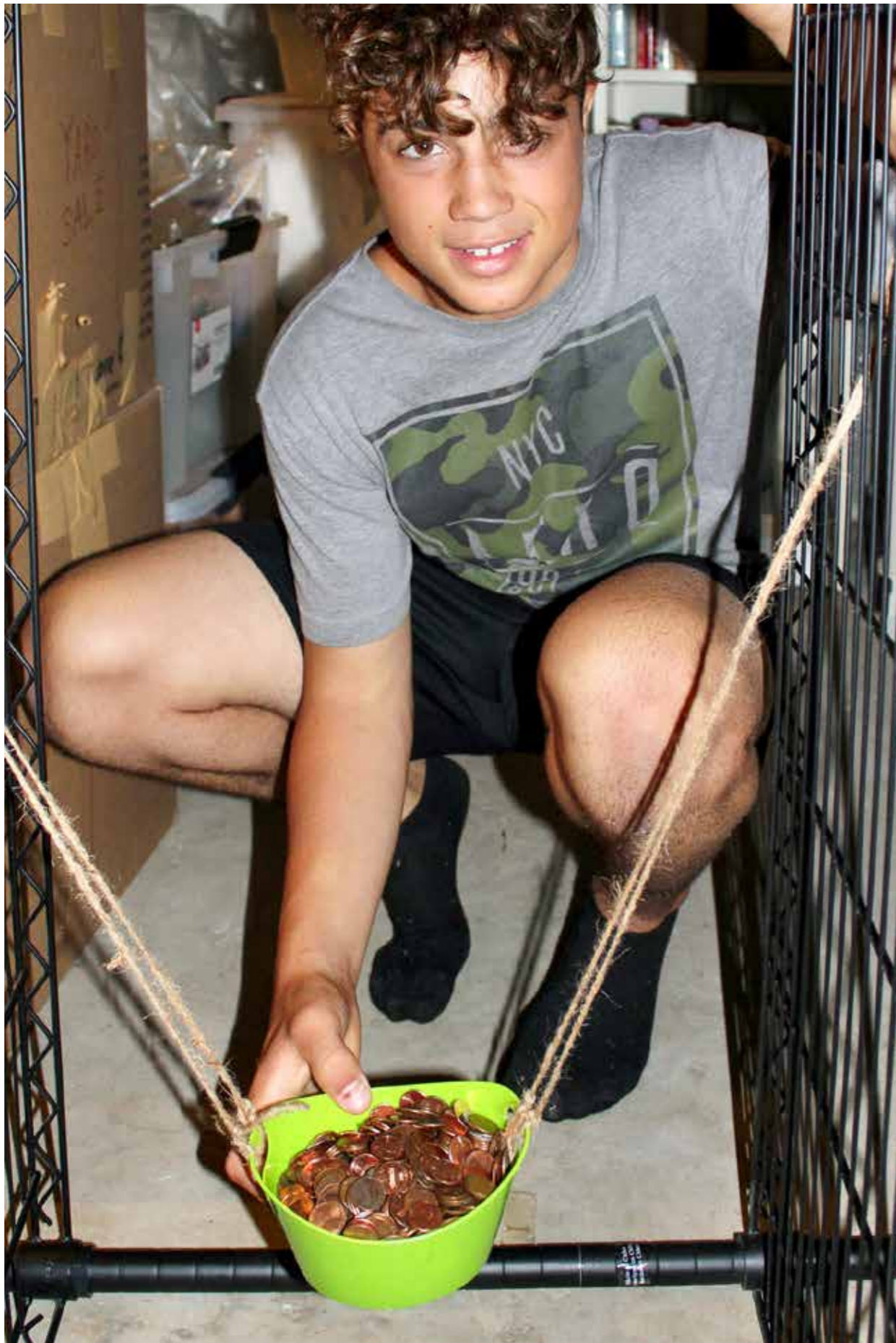
James, in Lt Col Maffei's basement, has reconfigured a shelving unit to test the adhesiveness of Derma-bond in test and control samples
